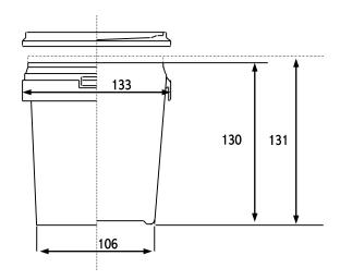
Measurements in millimetres
